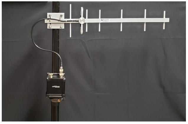
Single directional 9db Yagi antenna upgrade kit for use at the Fixed Master location. The kit is configured with one directional 9db antenna to extend the transmit range of the Fixed Master Outdoor Unit (ODU) in one direction away from the Fixed Master location. The kit includes one L-COM 9db Yagi antenna (HG909YE-NF) with pole mount (shown mounted on a customer provided ~2" pole dia.), one NF2NM cable adapter. STS-200-ODU (shown above) is not included in the kit.
