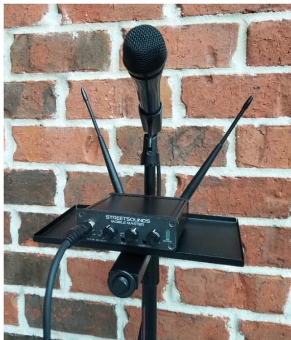
**NOTE: *If you do not have a microphone connected to the Mobi, make sure the Mic volume control is turned all the way down, otherwise you may experience noise and/or hum.***
