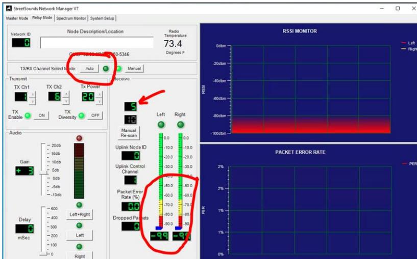
3. Turn on the Secondary Fixed Master Transmitter to the selected channel. To do this you may need to temporarily connect the NMS to the Secondary Master to properly configure its transmit channel.
