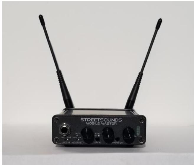
When using the Mobi for a street-side event, the roof-mounted Master is reconfigured to be a “repeater”. Thus, the Mobi talks to the repeater, and the repeater retransmits the signal to all the remotes. This means the Mobi does not have to cover the entire network from the ground.
